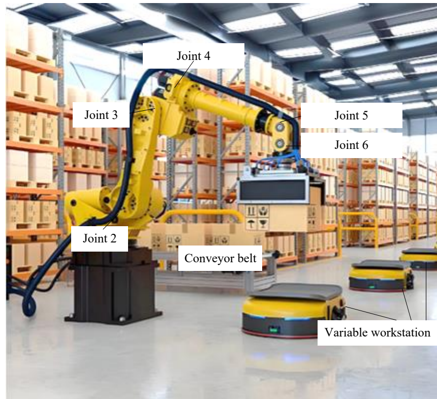
Figure 4. Actual working scenario of robotic arm.
